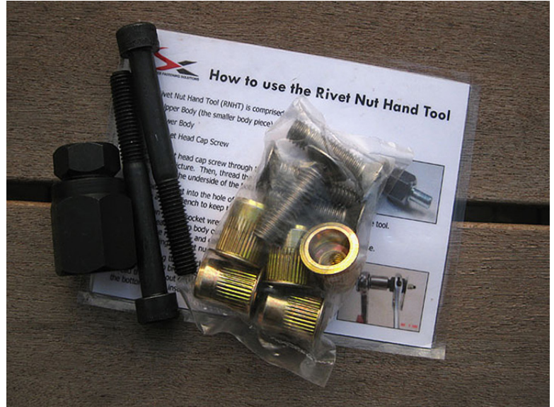
Recommended nutsert tool shown with stainless steel bolts and cad plated nutserts
